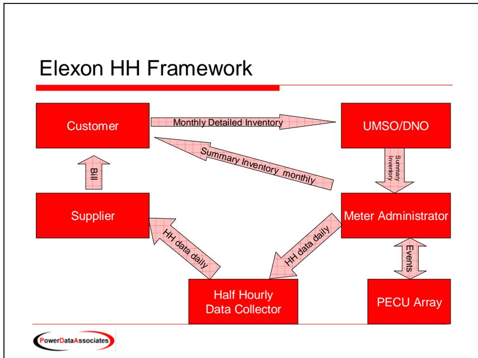
To accommodate the CMS data the interaction between Customer, UMSO and Meter Administrator have been modified.
